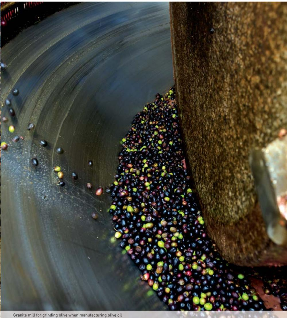
Granite mill for grinding olive when manufacturing olive oil
