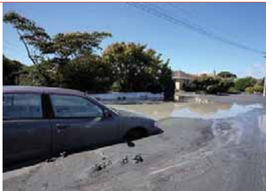
Figure 8: Liquefaction deposits in eastern Christchurch resulting from the 22 nd February. Christchurch earthquake. Removal of this material has resulted in a significant land level lowering with respect to sea level and the water table. (Photos: Tonkin & Taylor Ltd).
