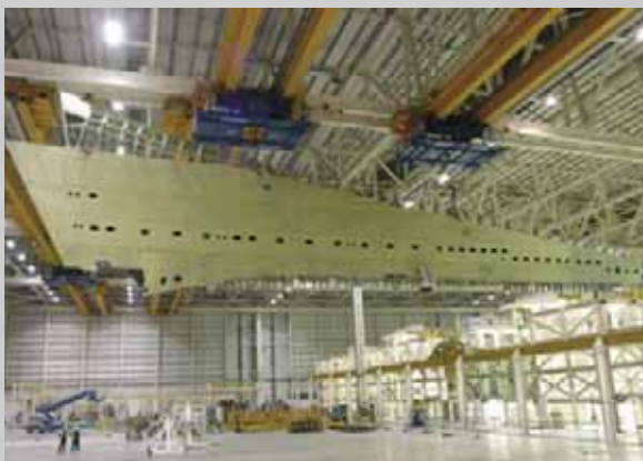
The first A380 wing was removed from its main assembly jig at Airbus' factory in Broughton, North Wales (UK) on November 4, 2003
