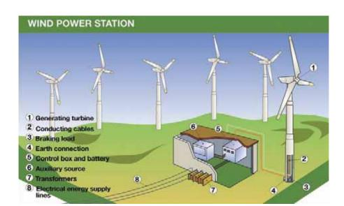
Wind energy is currently primarily used for the generation of electricity which is then sold to the national supply grid, this is done by installing a number of windmills in what is known as a wind farm.
